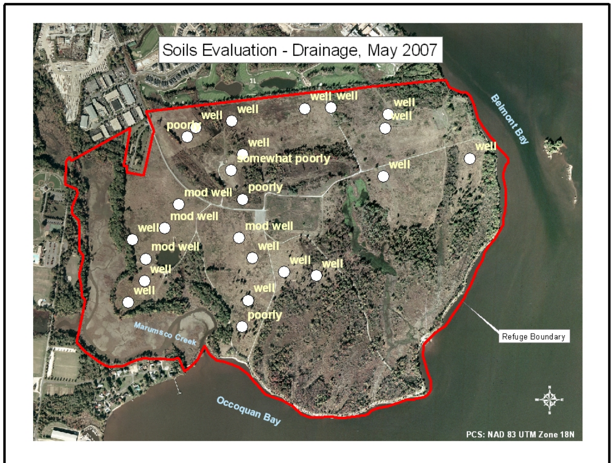
Figure 8. Soil borings at Occoquan Bay NWR, evaluated by NRCS, 2007.
