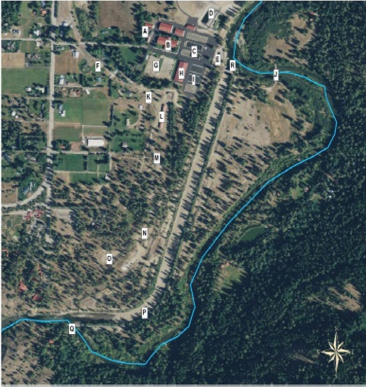
Figure B2. Aerial view of Leavenworth NFH and Icicle Creek (blue line). Letters denote hatchery infrastructure. Shallow wells (#1, 2, 3, and 7) are denoted by: M (Well 1), N (Well 2 and 7), and O (Well 3). Deep wells are denoted by A (Well 5), F (Well 6), and K (Well 4). The hatchery channel is labeled P and is dewatered in this image. The figure is adapted from Potter et al. (2017).
