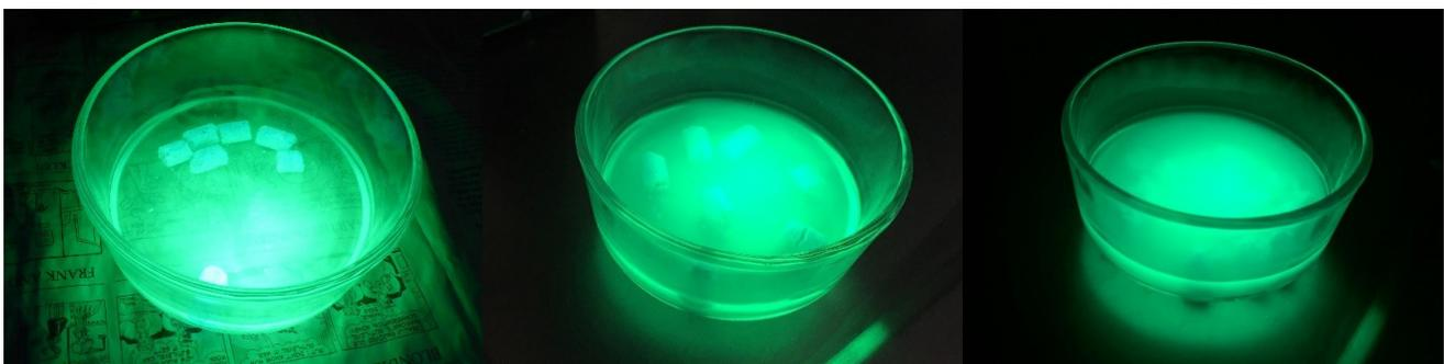
Figure 5: Pyranine fluorescence in solution. Six diphacinone pellets in tap water under UV lighting at 10 minutes (left), 24 hours (center), and 24 hours with water-softened pellets mashed to release interior pyranine solute.
