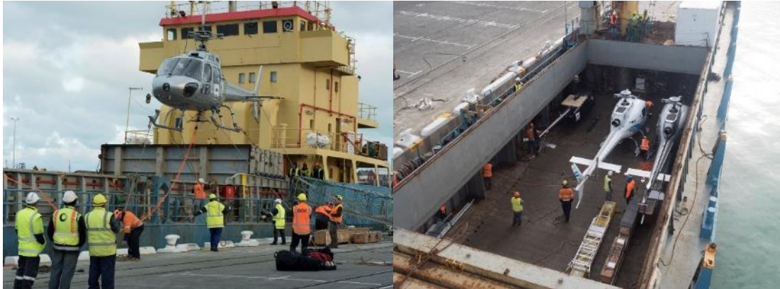
Figure 12: Loading helicopters from the wharf into the upper level of the Norfolk Guardian's hold
