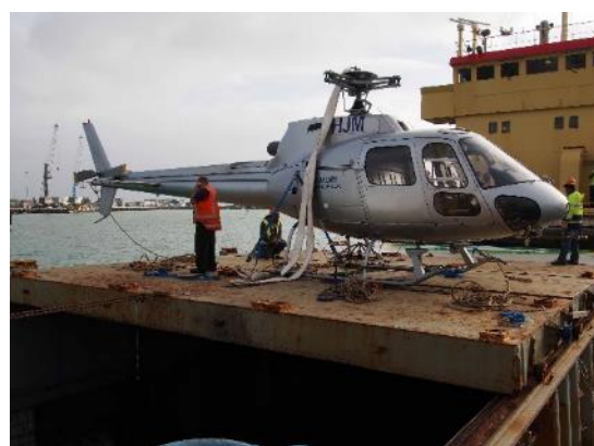
Figure 11: Helicopter placed on open hatch cover ready for the 2nd crane to pull the hatch closed.
