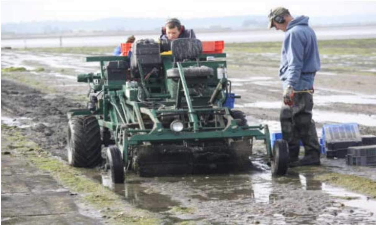
Figure 9. Mechanical clam harvester (Pacific Shellfish Institute 2015)
