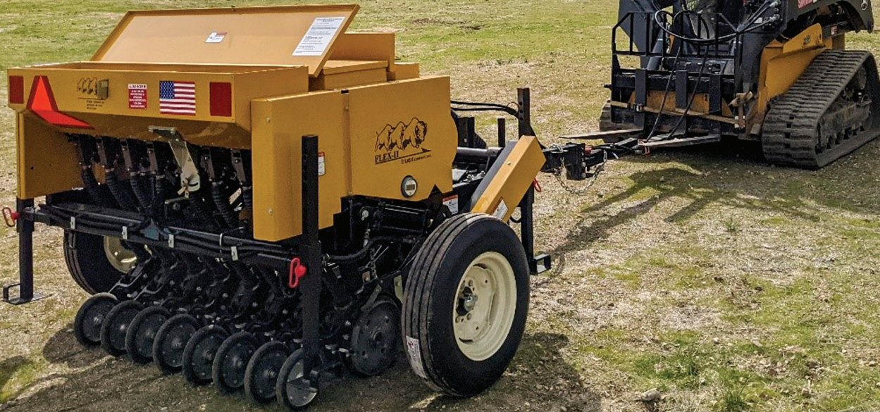
Drill seeders can put large amounts of seed into the ground quickly and consistently with minimal impact to the ground surface. At optimal capability, a drill seeder can travel 4 to 6 mph and seed about two acres of ground per hour. Courtesy Patrick Riparetti
